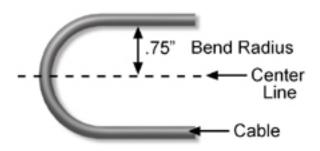
Bend Radius. What's the bend radius on your cabling? It's critical that you know this in order to ensure proper operation of the cable (i.e., optimal data flow-through). The bend radius is the distance between the center line of the bend to the inner edge of the parallel cable.
