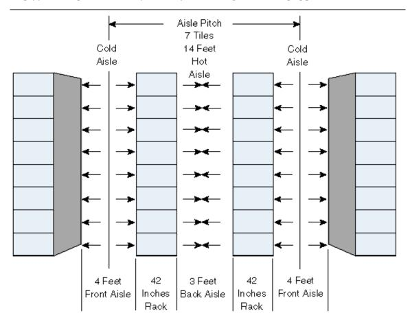
For server locations with multiple enclosures, providing adequate space around each of the units also ensures proper ventilation and air circulation. By providing adequate circulation, you keep the overall room temperature down which improves server efficiency and also makes your air conditioner work less to keep that temperature (which saves money as well).
